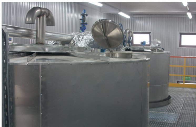
The new blending unit allows the company to compose a number of specialized industrial waxes with great precision
